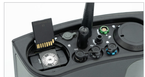
SD-card slot to simplify data sharing without connecting to the PC
