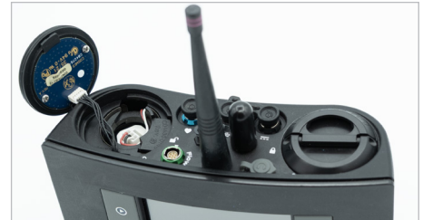
User replaceable O 2 sensor and/or battery; an easy operation not requiring special tools
